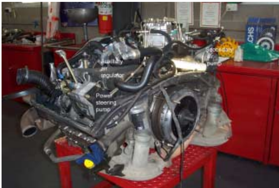
M30/69 turbocharged engine, image courtesy of Kevin Ross
