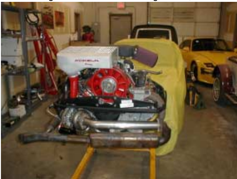
930/XX turbocharged engine. Photo by Stephen Kaspar.
