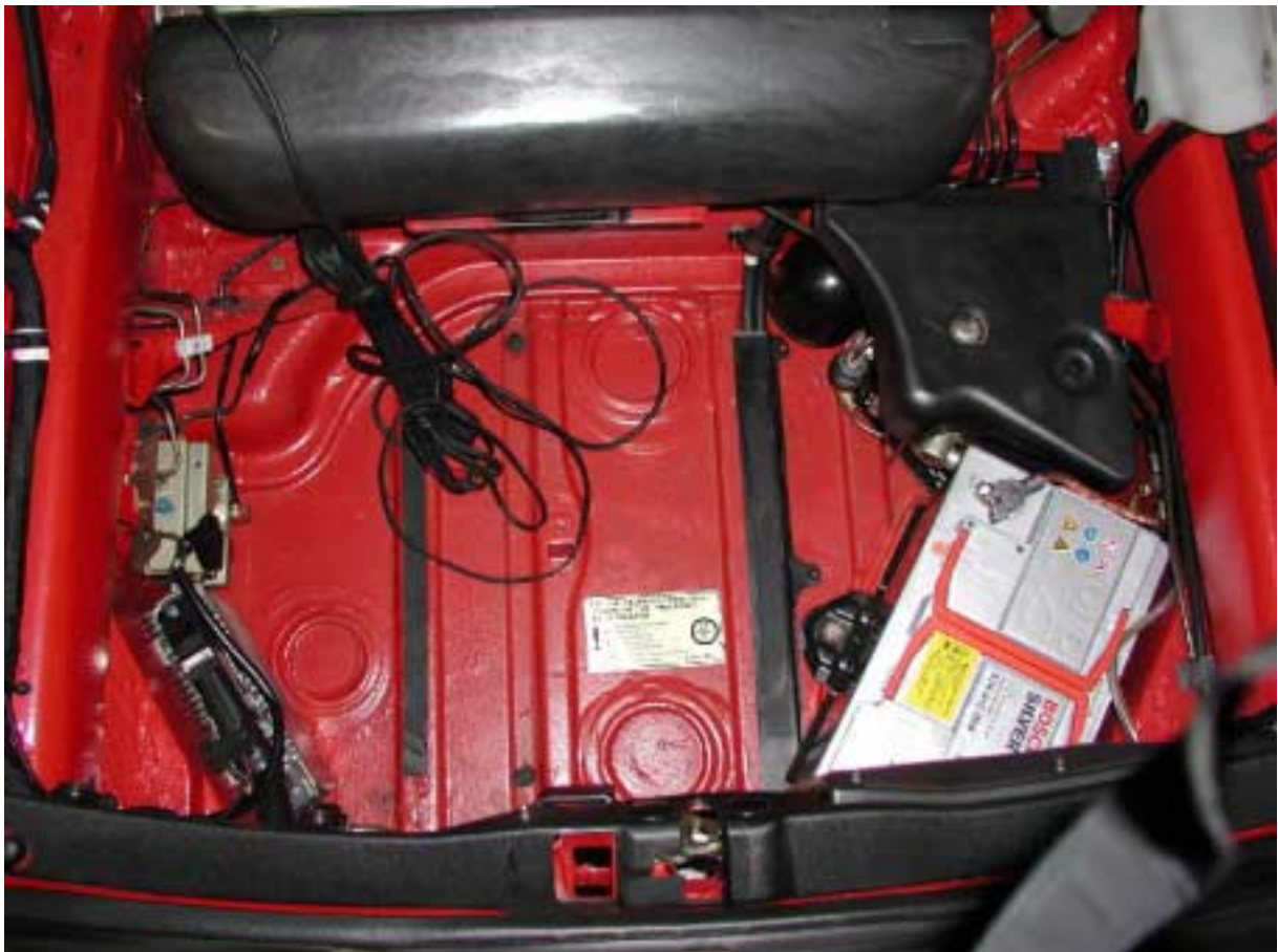
Component locations from left to right: PDAS/ABS control unit, differential lock dual solenoid valve, brake hydraulic boost pressure accumulator, ABS hydraulic unit. Photo by Yasutoshi Kikuchi
