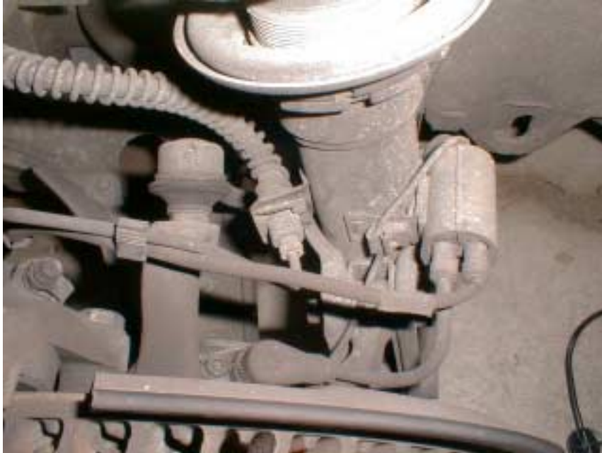
Wheel speed sensor with combination plug (noise suppressor) photo by Tom Sharpes
