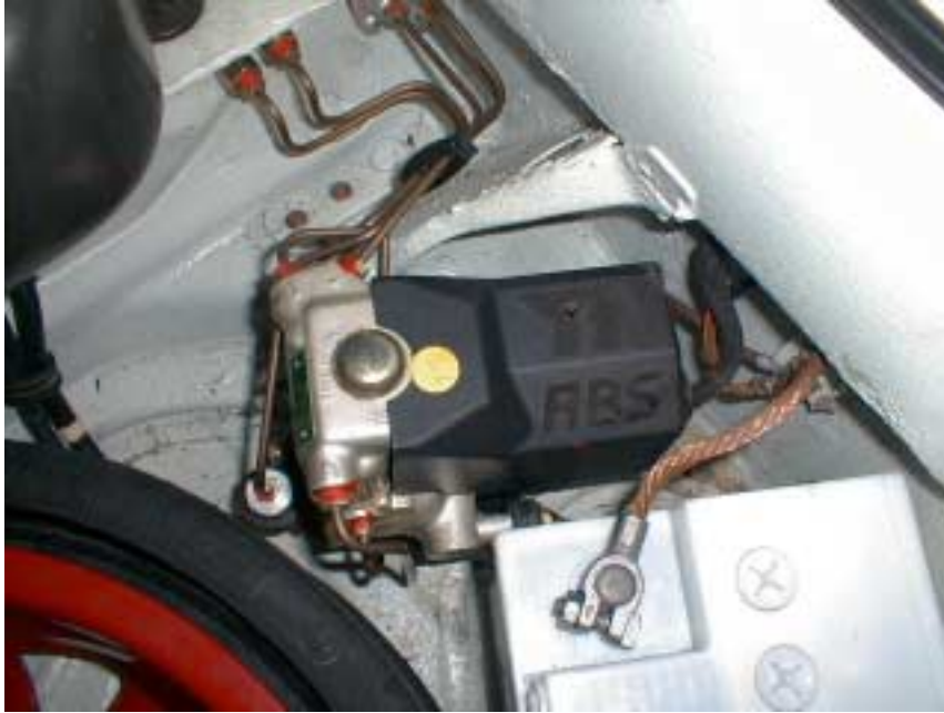
Carrera 2 ABS hydraulic unit. Photo by Tom Sharpes
