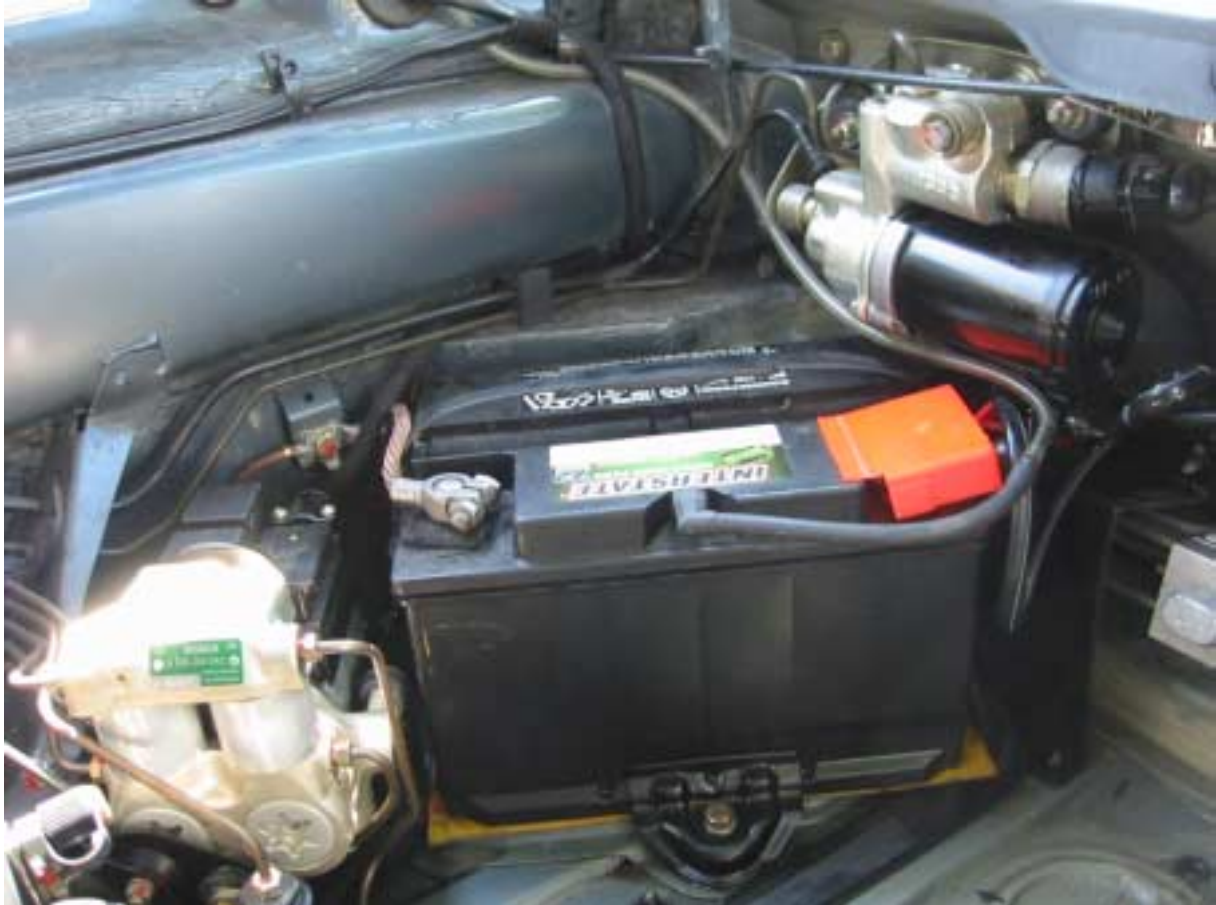
Component locations from left to right: ABS hydraulic unit, Battery, Brake hydraulic boost pump. Photo by Michael Wu.
