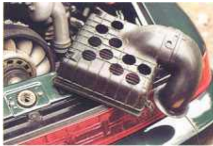
The airbox clips off and lifts out easily (top). Drilling large holes in the outer surface (above) increases induction roar and takes a matter of minutes (see text)
