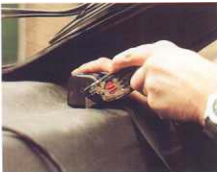
Rubber soundproofing had to be cut away to allow the inertia-reel units to be fitted – threaded mounting holes were underneath
