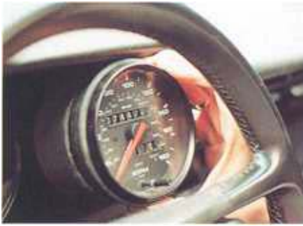
New speedometer simply pushes into the dash aperture and is very simple to fit, particularly when compared to doing the same job in, say, a 944 or Boxster
