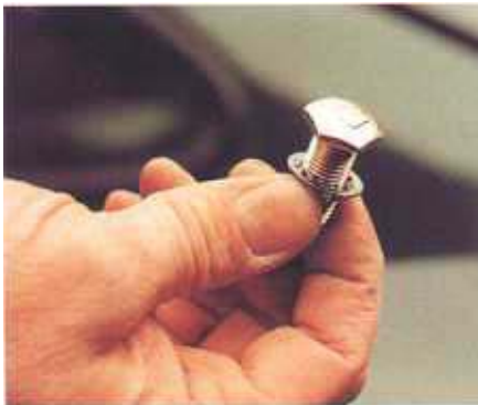
Brand-new, approved seat-belt mounting bolts and washers were used (see text)
