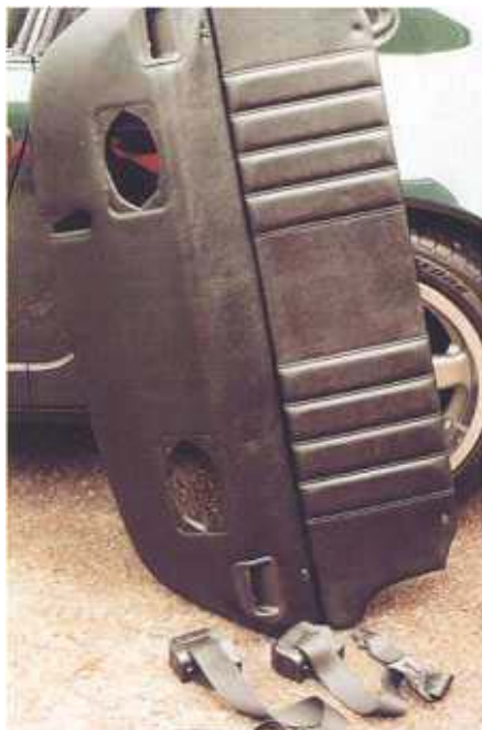
The parcel shelf is retained by four screws (above). Once these are removed – and the speaker wires disconnected – the panel can be lifted out quite easily
