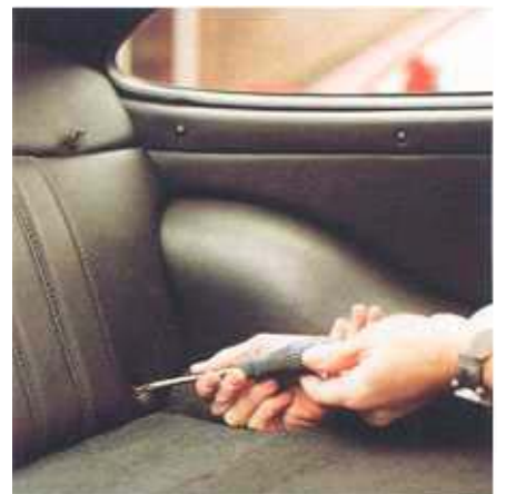
The parcel shelf is retained by four screws (above). Once these are removed – and the speaker wires disconnected – the panel can be lifted out quite easily
