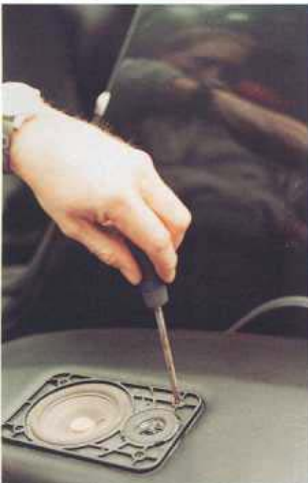
Loudspeaker covers prise off to reveal mounting screws. Speakers were then transferred to the new parcel shelf
