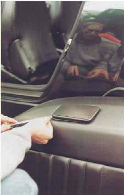
New speedometer simply pushes into the dash aperture and is very simple to fit, particularly when compared to doing the same job in, say, a 944 or Boxster
