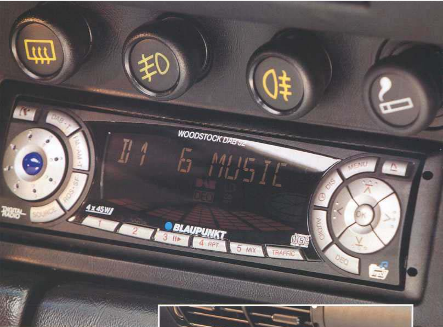
New Blaupunkt Woodstock DAB52 (above) fits in well with the 911 dashboard. Original unit (right) was also made by Blaupunkt, but technology has moved on in the last 13 years
