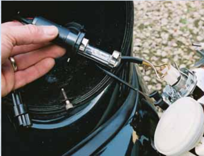
Xenon bulb assembly (in author's hand) is about 30mm too deep to fit inside the standard 964 headlamp bowl, and is substantially larger than the original halogen bulb, the rear of which you can see still installed here in the glass headlamp unit on the right
