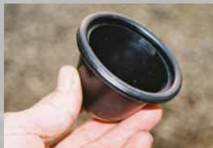
Rubber cap from the rear damper from a Mark I Golf is ideal for creating (dry) extra space at rear of headlamp bowl in order to accommodate special xenon bulb
