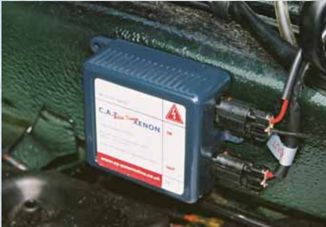
Ballast boxes (left) fitted inside the luggage compartment and were neatly covered by the loose-fitting carpet (right)
