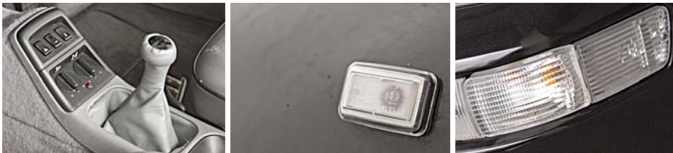
New gear lever gaiter was awkward to fit and finish is not up to standard. New clear side repeaters and indicator lenses help lift 964's classics looks. All parts supplied by Porscheshop (details above).
